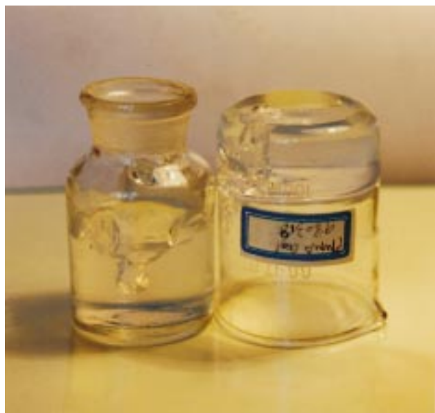
Figure 1. A picture of nearly transparent polymeric hydrogels: left, PMMA-980317; right, PMMA-980318.
